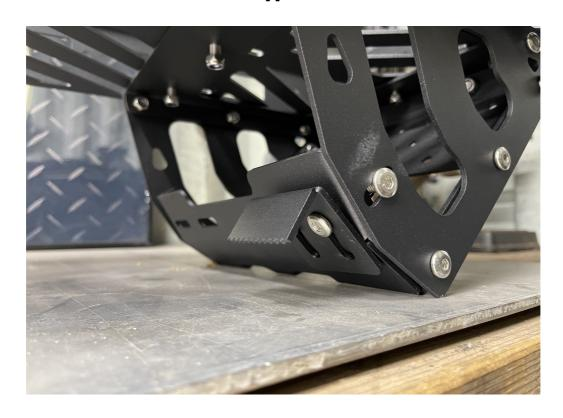
Set the rack on the spare tire and adjust the side panels in to where they are touching the tire firmly and tighten all hardware.
