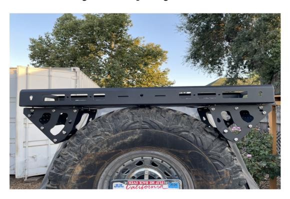
Attach the provided ratchet straps as show and feed them through the holes in the wheel and tighten. Note some adjustment may be needed at this time to ensure the rack sits level and secure.
